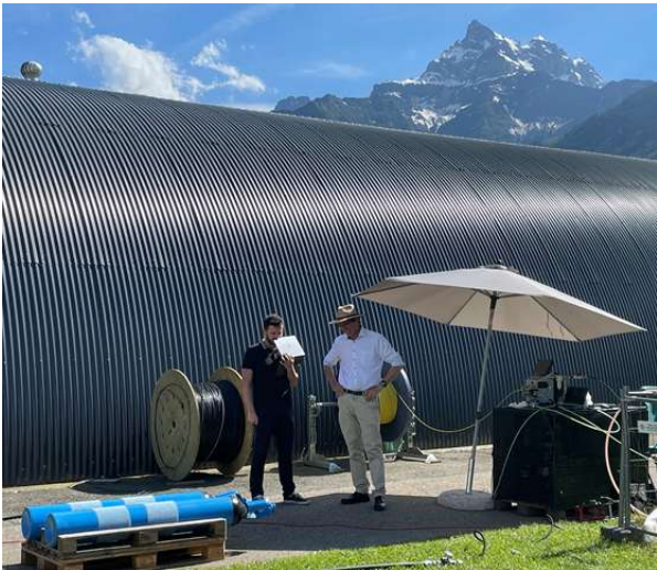
Figure 16. Test setup with pressure controlled blowing machine and flow measurements, using gas cylinders
